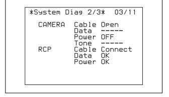
**CAMERA cable:** Camera cable connection status (connected/shorted)
